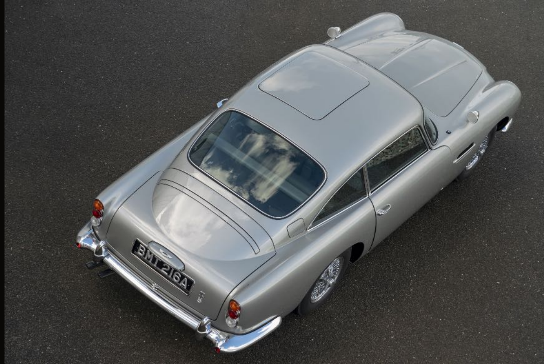
The cars will feature original DB5 styled aluminium exterior body panels on an authentic DB5 mild steel chassis. Under the bonnet is a 4 litre six cylinder naturally aspirated engine with three SU carburettors and an oil cooler, which produces 290 bhp. Attached to a 5 speed ZF manual gearbox with a rear mechanical limited slip differential.
