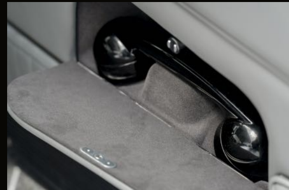
Telephone in driver's door.
