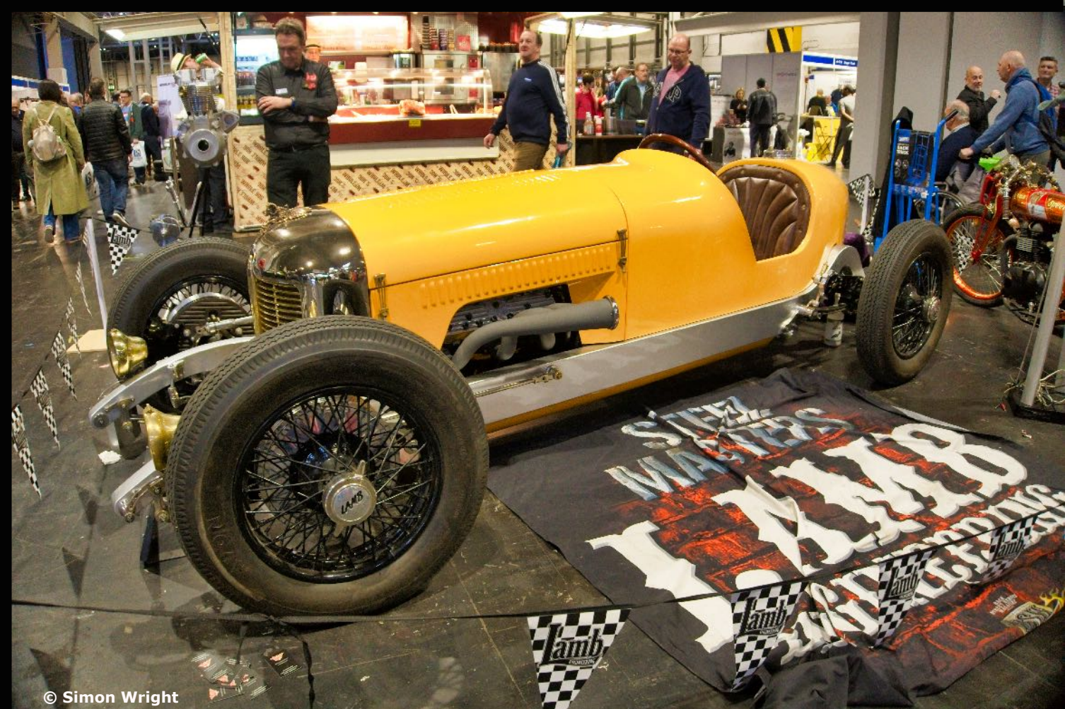
The Craftsman built by Lamb Engineering as a tribute to the Miller V8 Indianapolis car of the 1920s. This has a French Flathead V8 engine/
