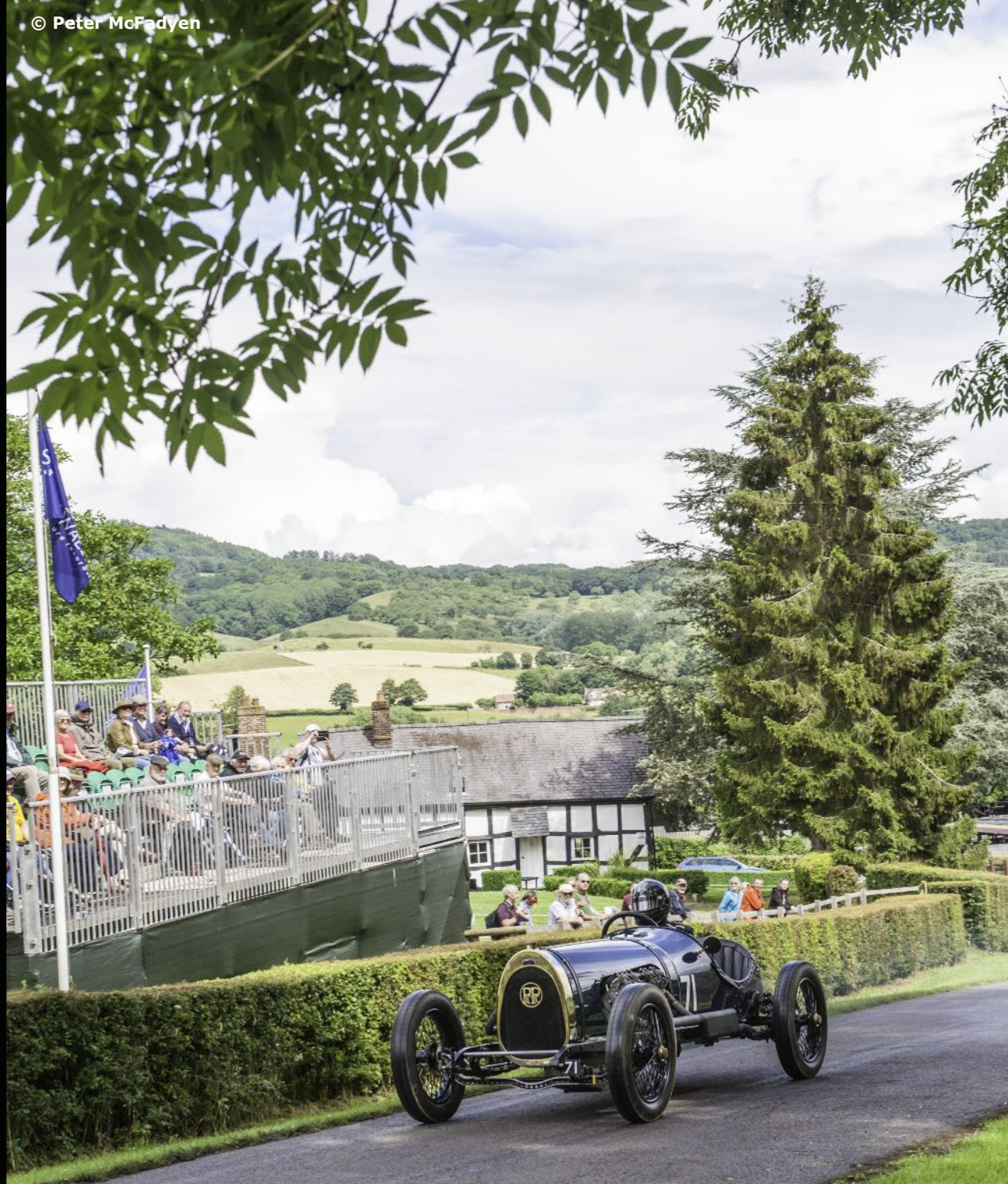
Geoff Smith's Piccard Pictet Special is powered by a nine litre Sturtevant Aero engine
