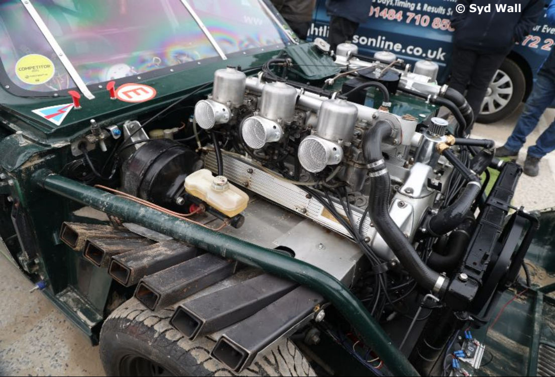
A one-off 8.73 litre Quad Cam V12 engine. Two straight six Jag engines mounted on a common crankcase.
