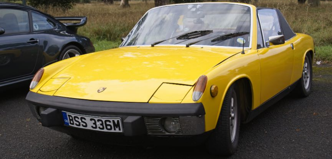
1973 Porsche 914 mid-engined sports car produced between 1969 and 1976. Powered by a 2 litre flat 4 boxer engine producing 99 hp, giving a top speed of 118 mph and do 0-62 mph in 10.5 seconds.
