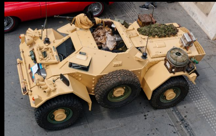
1959 Daimler Ferret Armoured Scout car with a Rolls Royce B60 engine
