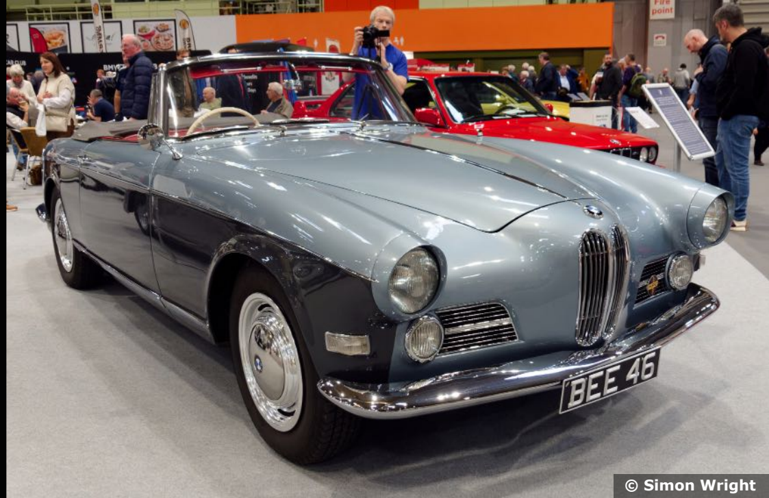
Ex John Surtees 1957 BMW 503 Cabriolet. One of only 3 RHD 503 Cabriolets custom built by BMW. The all alloy 3.2 litre V8 engine was a World first. It produced 150 bhp, giving a top speed of 125 mph. It was on the BMW Historic Motor Club stand.
