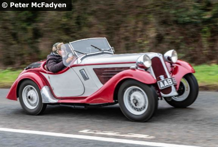
A 1936 Rover 12HP open 4-seater for which the first owner paid £288. It has a 4-cylinder 1496cc OHV engine and features included Bijur automatic chassis lubrication
