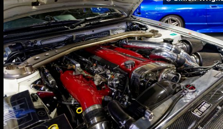
2.8 litre engine from a 2000 Nissan GT-R
