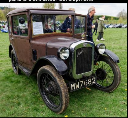
1928 Austin 7. RK Fabric saloon built at Longbridge. 750cc side-valve engine. Top speed 55 mph.
