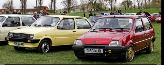
The Austin Mini Metro 1.3 HLS was a modern hatchback design to replace the Mini, using the same A Series FWD engine and transmission. The Rover Metro was launched in 1990 with the new K-Series engine of 1.1 or 1.4 litre. In some markets it was sold as the Rover 100 Series, with the Rover 111 and the Rover 114.
