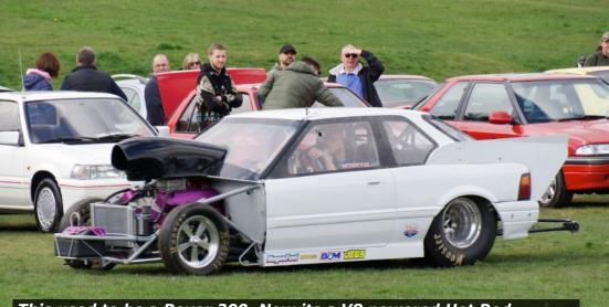
This used to be a Rover 200. Now its a V8 powered Hot Rod, producing 1100 bhp normally aspirated and 1600 bhp on Nitro. Driven by Maek Beswick.
