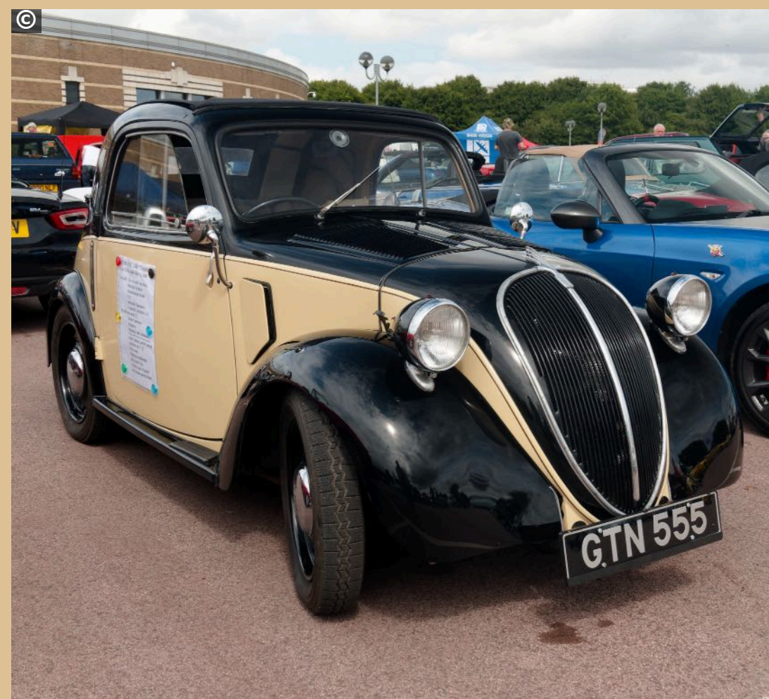
1938 Fiat 500 Topolino Over 500,000 were built between 1936 and 1955. Powered by a 570cc 4 cylinder side valve water cooled engine which produces 13 bhp. This gives a top speed of 53 mph and it could achieve 39 mpg. It had a 4-Speed manual gearbox with synchro on 3rd and 4th.
