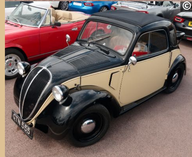
1938 Fiat 500 Topolino Over 500,000 were built between 1936 and 1955. Powered by a 570cc 4 cylinder side valve water cooled engine which produces 13 bhp. This gives a top speed of 53 mph and it could achieve 39 mpg. It had a 4-Speed manual gearbox with synchro on 3rd and 4th.
