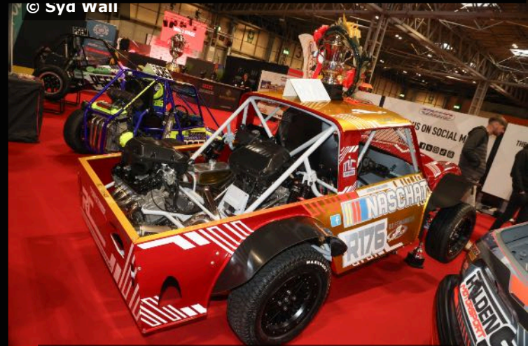
Twin bike engines in Autograss racer Julie Hawthorn-Fernihough's 2023 Class 7 winning Mini Pickup
