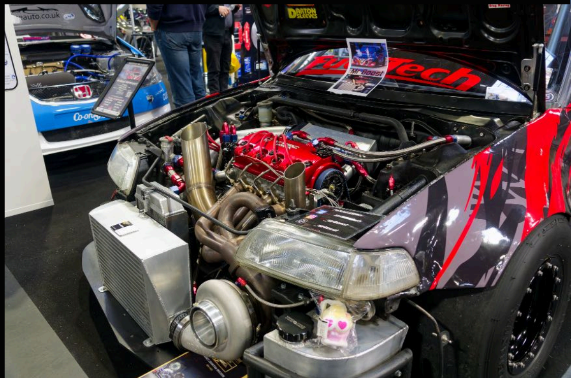
Mr Boost - Honda Civic FWD 1600 D Series engine turbocharged to 915 bhp. 9.1 secs 1/4 mile 161 mph Fastest D Series in Europe
