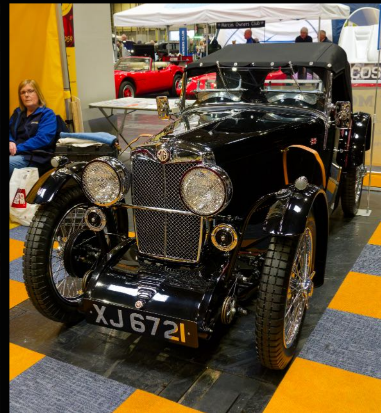
1933 MG J2 Midget. On the Owen Motoring Club stand was a 1933 MG J2 Midget. Over 2000 were built between 1932 and 1934 and cost £199 10s. It was powered by a 847cc engine derived from A Wolseley unit. It developed 36 bhp and gave a top speed of 80 mph
