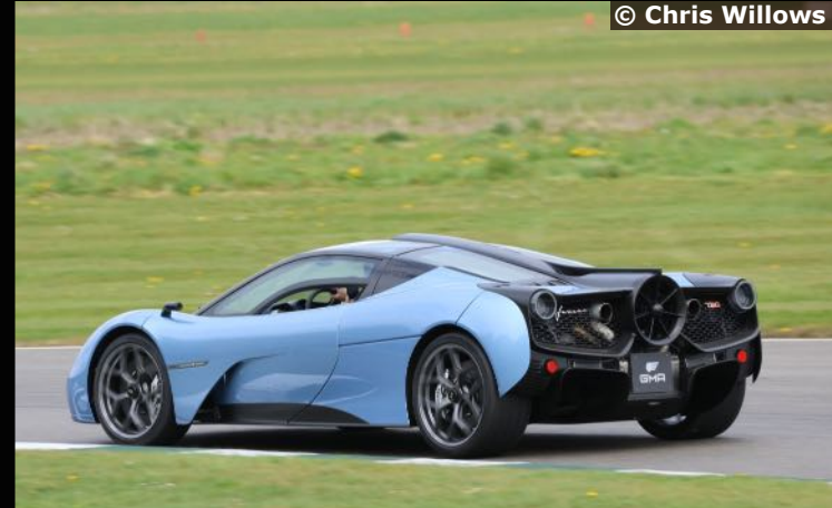
GMA T50 Rear View with Fan Helping Downforce
