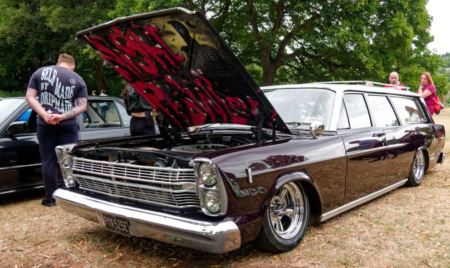
**1967 Ford Galaxie Ranch Wagon - Huxley Motorsport build 2019. Powered by a BMW 330D M57 Diesel engine (200 hp) & Automatic gearbox. Also has Toyota Supra front suspension.**
