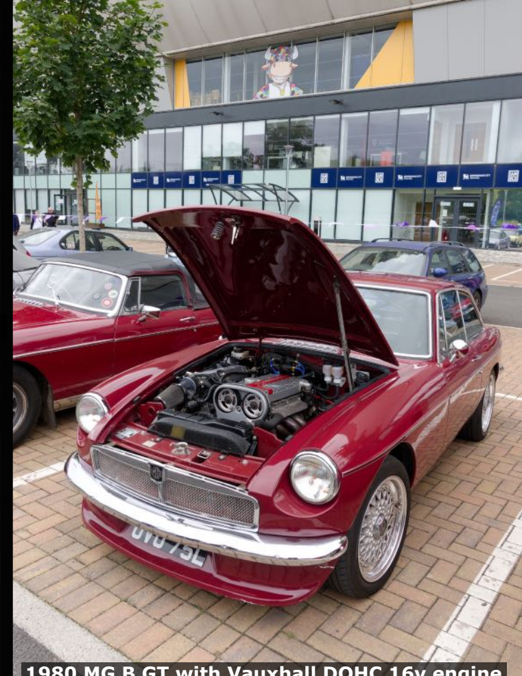
1980 MG B GT with Vauxhall DOHC 16v engine
