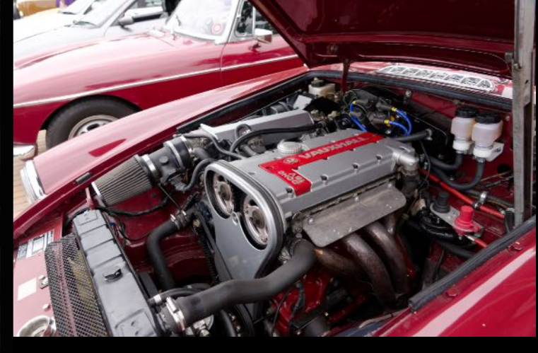
1980 MG B GT with Vauxhall DOHC 16v engine
