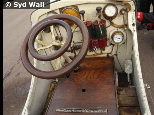
The controls of the White steamer, known as Whistling Billy, built by a sewing machine company
