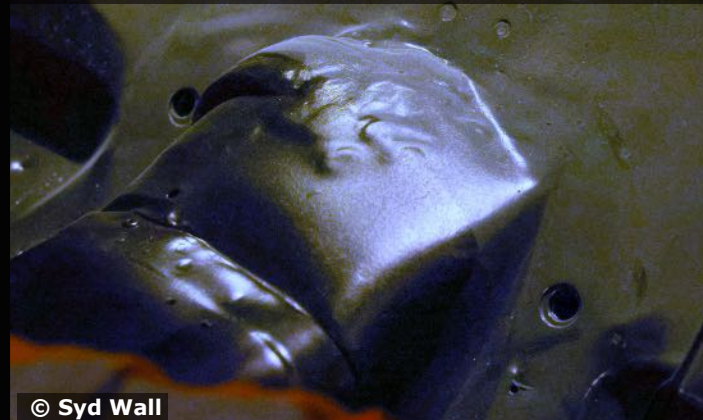
The transmission tunnel still shows the damage from the Ken Dawes prop shaft failure
