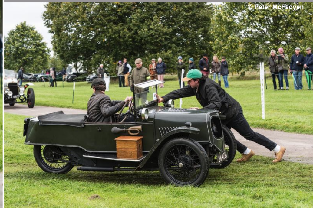
Cars without a reverse gear such as James Edwards' Morgan Sports Family Model are allowed to have a 'pusher' where a test involves going backwards
