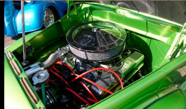
A more unusual car on display at Warwick was a 1947 Morris 8 Series E in a very bright metallic green paint job. It looked fairly normal externally but under the bonnet was a 3.9 litre Rover V8 engine.
